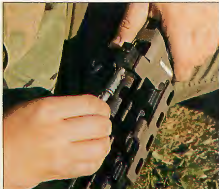
7 To strip the gas parts at the front of the SA80, lift the cover and pull the piston back so that the spring is depressed, and pull off the gas cylinder.
